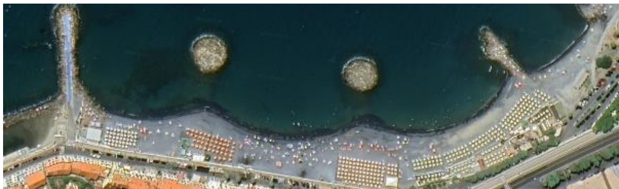
Figure 17. Offshore island for coastal erosion combined with groynes. Liguria, Italy. Credit: Google Earth.
