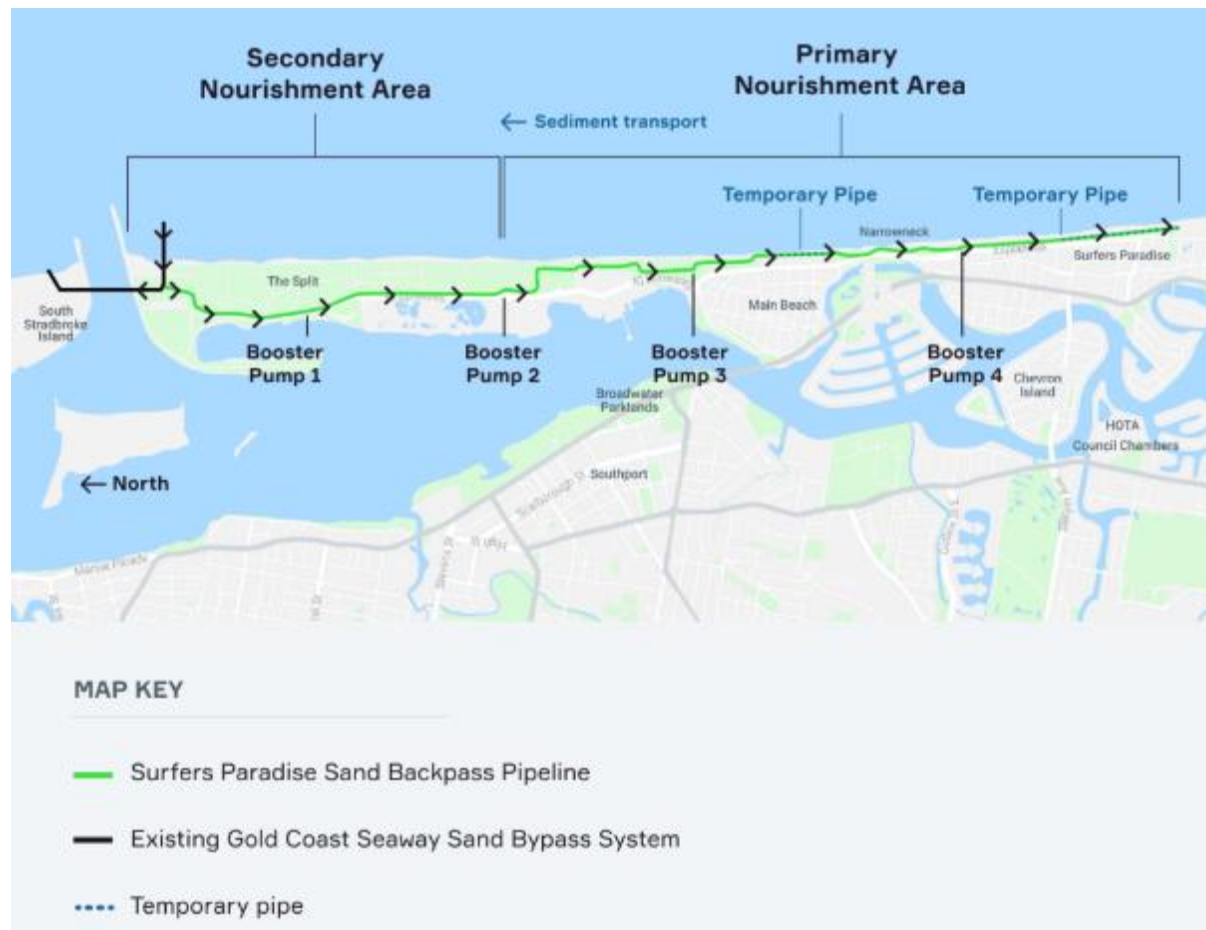
Figure 4. Surfers Paradise sand backpassing system scheme. The sand is captured by the Gold Coast Seaway jetty system and pumped back to Surfers Paradise approximately 4 km south. Credit: City of Gold Coast.
